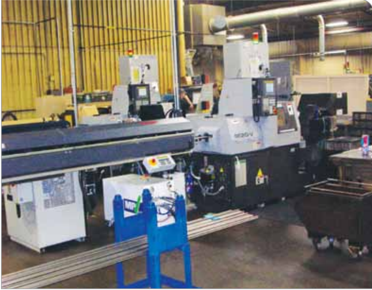
∴ The growing CNC Swiss department at Precision Metal has helped this screw machine shop grow its business without impacting the work performed on its multi-spindles.
