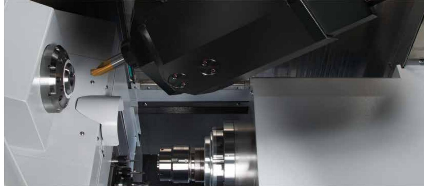
Productive combined machine by the integration of Swiss type automatic lathe (sliding headstock type) and machining center
