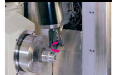
The tool can be indexed at fixed positions in 90 deg steps (4 positions) and tools can be used efficiently.
